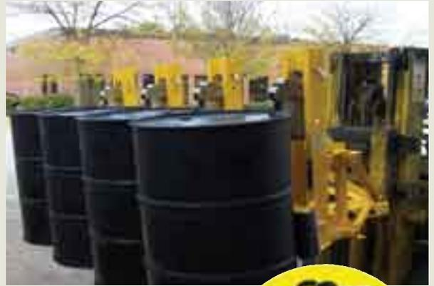
No Frills. No Bells. No Whistles. The FTA drum handling attachment for steel drums is just safe, solid, and basic drum handling. The same unit can also handle plastic and fiber drums, including the ISO drum.
